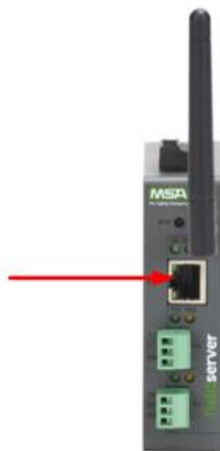
Figure 3-4: ProtoAir Ethernet TCP/IP and BACnet IP Connection
